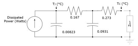
Note: ZEXT are the external thermal impedances (case to sink, sink to ambient, etc.). Set to zero when modeling only the case to junction.
