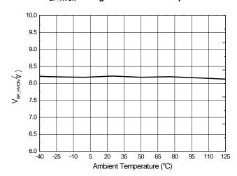
$V_{\mbox{\footnotesize{BP\_HVOFF}}}$  Voltage vs. Ambient Temperature
