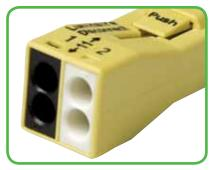
Molded in color coding for circuit wiring: Black = L White = N Red = dimming and switching (3-pole) Green = Ground (3-pole) Inkjet marking for additional requirements
