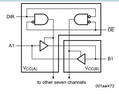
Fig. 2. Logic diagram (one channel)
