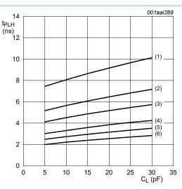
b. LOW to HIGH propagation delay (A to B)
