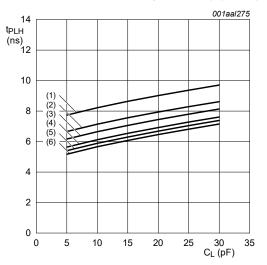
Fig. 10. Typical propagation delay versus load capacitance;  $T_{amb}$  = 25 °C;  $V_{CC(A)}$  = 1.5 V
