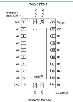
(1) This is not a ground pin. There is no electrical or mechanical requirement to solder the pad. In case soldered, the solder land should remain floating or connected to GND.
