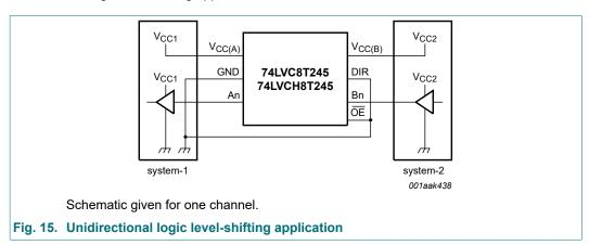
Table 15. Description unidirectional logic level-shifting application
