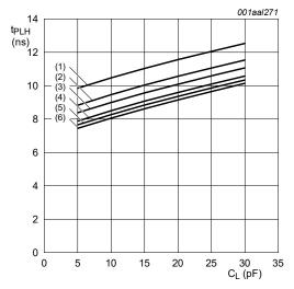
Typical propagation delay versus load capacitance;  $T_{amb}$  = 25 °C;  $V_{CC(A)}$  = 1.2 V
