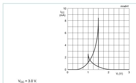
Fig. 10. Typical transfer characteristics
