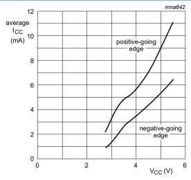
Linear change of V<sub>I</sub> between 0.8 V to 2.0 V.
