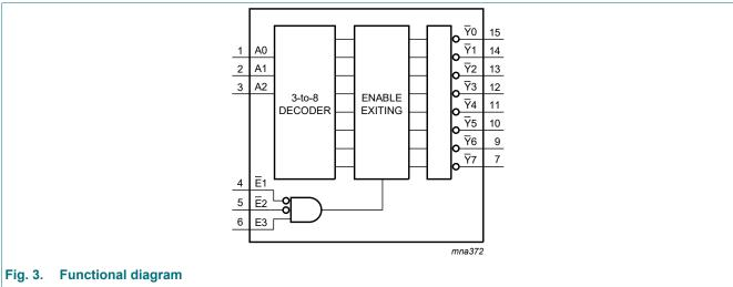
3-to-8 line decoder/demultiplexer; inverting
