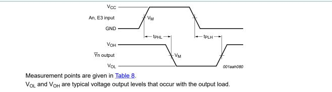
Fig. 7. The inputs An, E3 to outputs  $\overline{Y}n$  propagation delays
