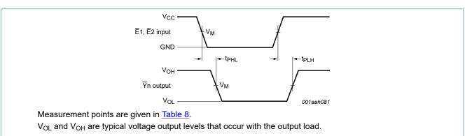
Fig. 8. The inputs  $\overline{E}$ n to outputs  $\overline{Y}$ n propagation delays
