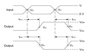
**Voltage Waveform** Propagation Delay Times
