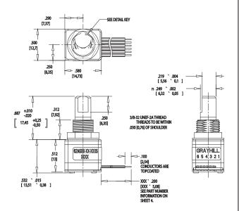
S - .050 Center Ribbon Cable with .100 stripped end
