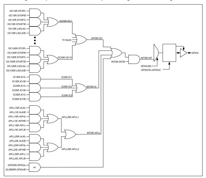
Figure 13 - Interrupt Structure
