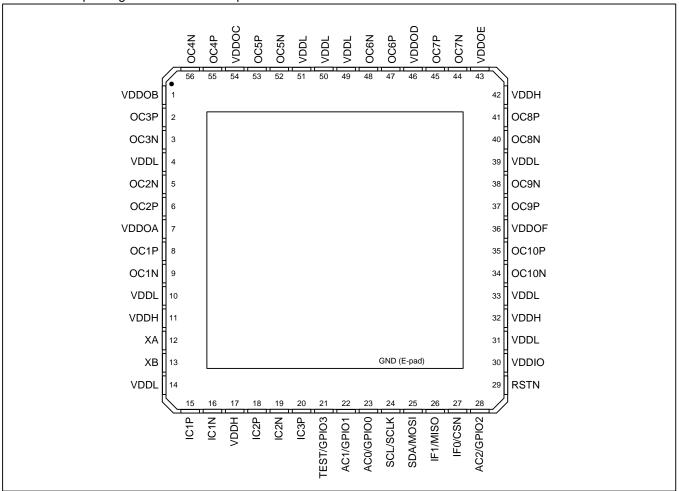
Figure 3 - Pin Diagram
