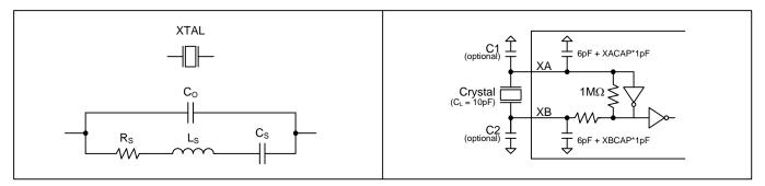
Figure 4 - Crystal Equivalent Circuit / Recommended Crystal Circuit
