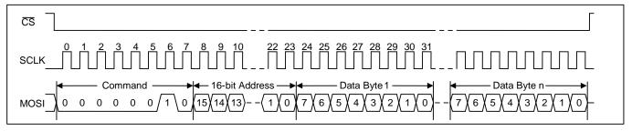
Figure 8 - SPI Write Transaction Functional Timing
