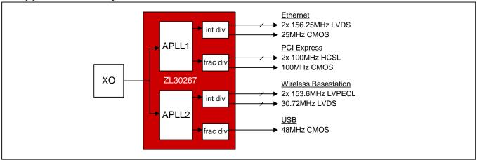
Figure 2 - Application Example: ZL30267 Ethernet, PCle, Wireless and USB Clocks Simultaneously
