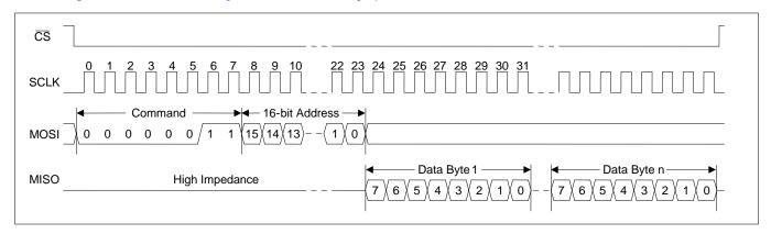
Figure 6 - SPI Read Transaction Functional Timing
