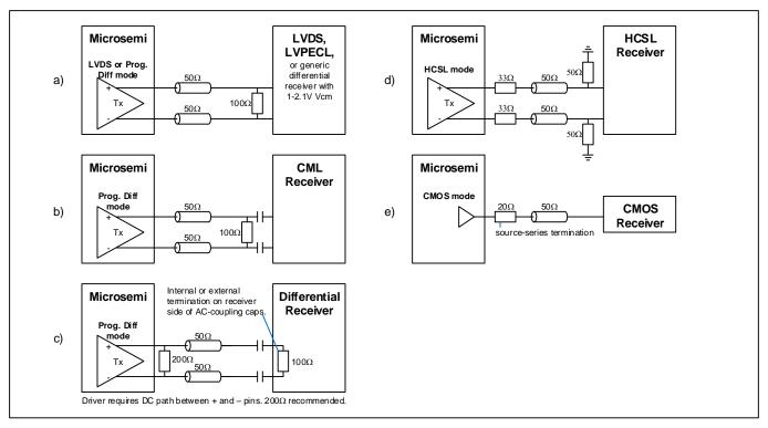
Figure 17 - Example External Components for Output Signals
