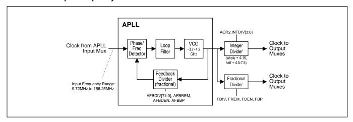
Figure 5 - APLL Block Diagram
