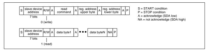
Figure 9 - I<sup>2</sup>C Read Transaction Functional Timing
