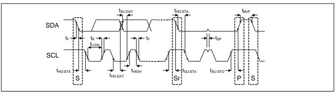
Figure 20 - I<sup>2</sup>C Slave Interface Timing
