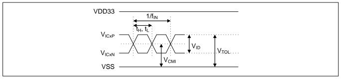
Figure 14 - Electrical Characteristics: Clock Inputs
