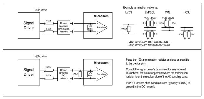
Figure 15 - Example External Components for Differential Input Signals
