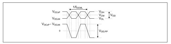
Figure 16 - Electrical Characteristics: Differential Clock Outputs
