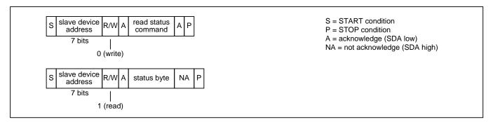
Figure 12 - I<sup>2</sup>C EEPROM Read Status Transaction Functional Timing (ZL30265 and ZL30267 Only)
