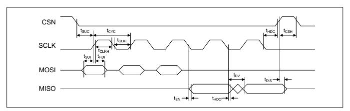
Figure 18 - SPI Slave Interface Timing
