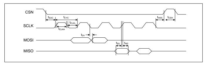
Figure 19 - SPI Master Interface Timing
