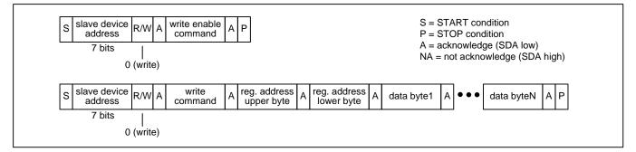
Figure 11 - I<sup>2</sup>C EEPROM Write Transaction Functional Timing (ZL30265 and ZL30267 Only)
