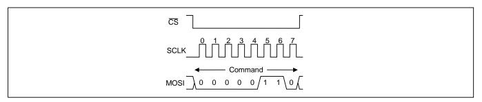
Figure 7 - SPI Write Enable Transaction Functional Timing (ZL30265 and ZL30267 Only)
