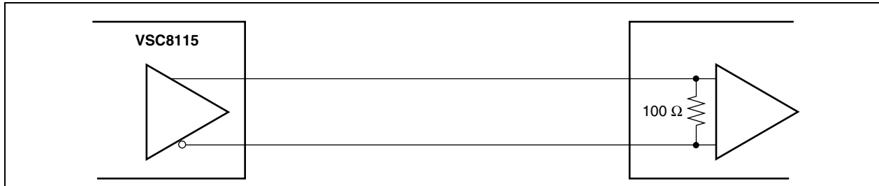
Figure 4. High-Speed Outputs, LVDS Termination
