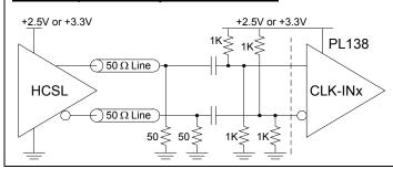
HCSL presents its signals very close to the ground rail, below the  $V_{\text{CMR}}$  range, so the HCSL signals can not be connected to the PL138 input directly. AC coupling is required for HCSL signals on the PL138 input.
