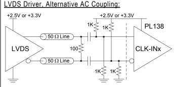
This circuit is for compatibility only. AC coupling is not really required for LVDS. The  $V_{\text{CMR}}$  range of the PL138 reaches low enough that LVDS signals can be connected directly to the PL138 input like in the circuit to the left.
