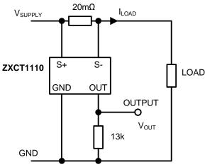
Figure 3 Example Circuit using ZXCT1110Q
