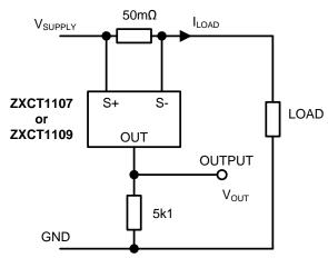
Figure 2 Example Circuit using ZXCT1107Q/09Q
