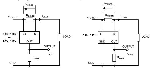
**Figure 1 Basic Application Circuit**
