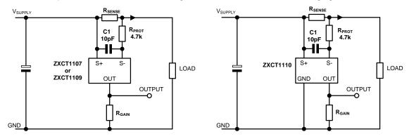
Figure 4 Protection and EMC Filtering
