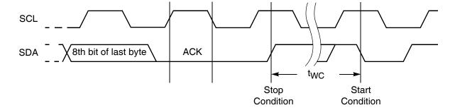
Figure 25. Write Protect (WP) Pin Timing During Slave Address
