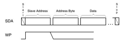
Figure 27. DCP "Wiper Position" Timing
