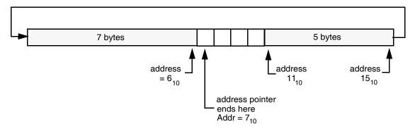
Figure 13. Example: Writing 2 bytes to a 16-byte page starting at location 11.
