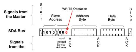
Figure 11. EEPROM Byte Write Sequence
