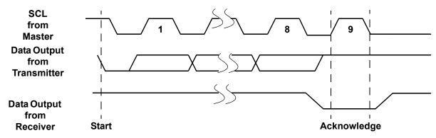
Figure 3. Acknowledge Response From Receiver
