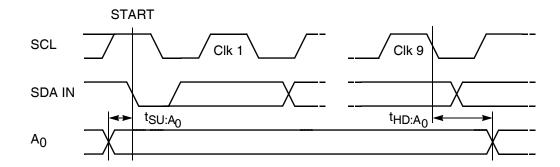
Figure 24. Write Cycle Timing
