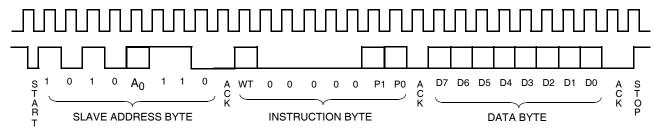
Figure 9. DCP Write Command Sequence
