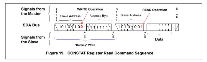
CONSTAT register. A write to the CONSTAT register itself, further requires the setting of the RWEL bit. Block Lock protection of the device enables the user to inhibit writes to certain regions of the EEPROM memory, as well as to all the DCPs. One further level of data protection in the X9525, is incorporated in the form of the Write Protection pin.
