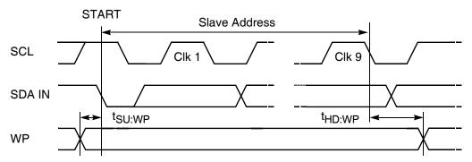
Figure 26. Write Protect (WP) Pin Timing
