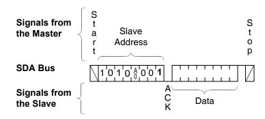
Figure 15. Current EEPROM Address Read Sequence
