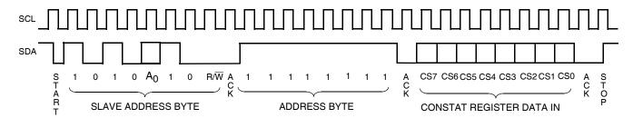
Figure 18. CONSTAT Register Write Command Sequence
