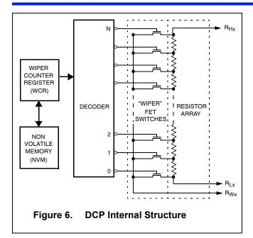
values of the DCP WCR's (before the contents of the NVM is loaded into the WCR) are 0 and 255 for DCP1 (100 tap) and DCP2 (256 tap) respectively. The data in the WCR is then decoded to select and enable one of the respective FET switches. A "make before break" sequence is used internally for the FET switches when the wiper is moved from one tap position to another.
