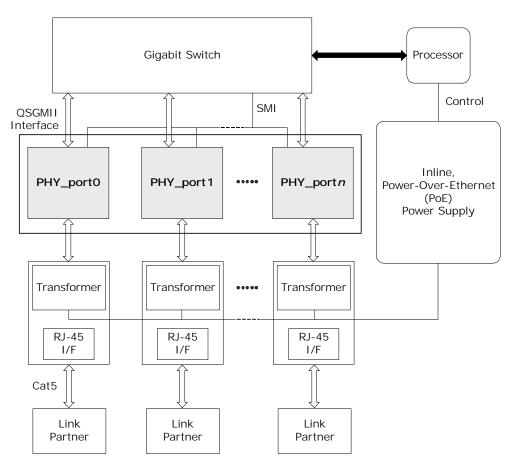
The following procedure describes the process that an Ethernet switch must perform to process inlinepower requests made by a link partner that is, in turn, capable of receiving inline-power:
