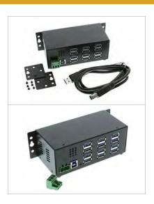
The Super-Speed 12-Port USB 3.0 Powered Hub is backward compatible with USB 2.0 and 1.1 specifications. It provides an out of the box industry standard that allows connection of up to twelve USB peripherals or devices to your PC or Mac USB ready host. The USBG-12U3ML 12-Port USB 3.0 Powered Hub is targeted at Industrial Application users for both PC and Mac that are expanding the number of USB ports on their system.
