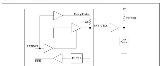
FIGURE 8-3: PORT POWER CONTROL USING A POLY FUSE
