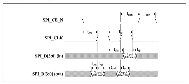
TABLE 9-7: SPI/SQI MASTER TIMING (30 MHZ OPERATION)
