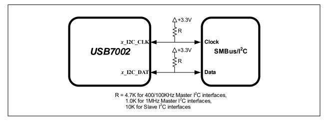
**Note:** Resistor values detailed in Figure 4-3 are suggestions. Optimal pull-up values may vary dependent on external factors.
