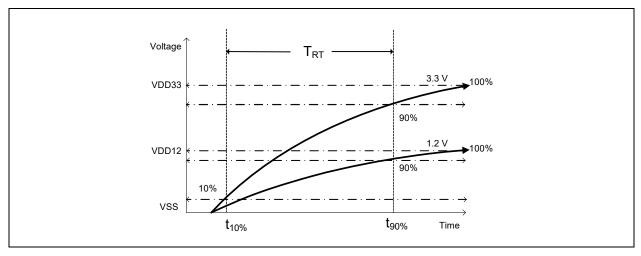
**Note:** The Power Supply Rise time requirement does not apply if the RESET\_N signal is held low during power on and released after power levels rise and stabilize above the power on thresholds, or if the RESET\_N signal is toggled after power supplies become stable.
