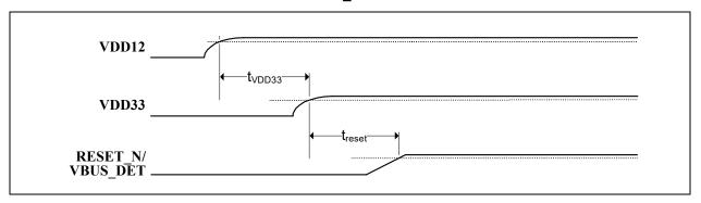
TABLE 9-4: POWER SUPPLY AND RESET\_N SEQUENCE TIMING
