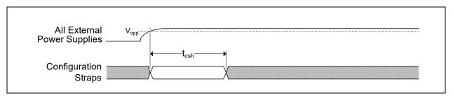
TABLE 9-5: POWER-ON CONFIGURATION STRAP LATCHING TIMING
