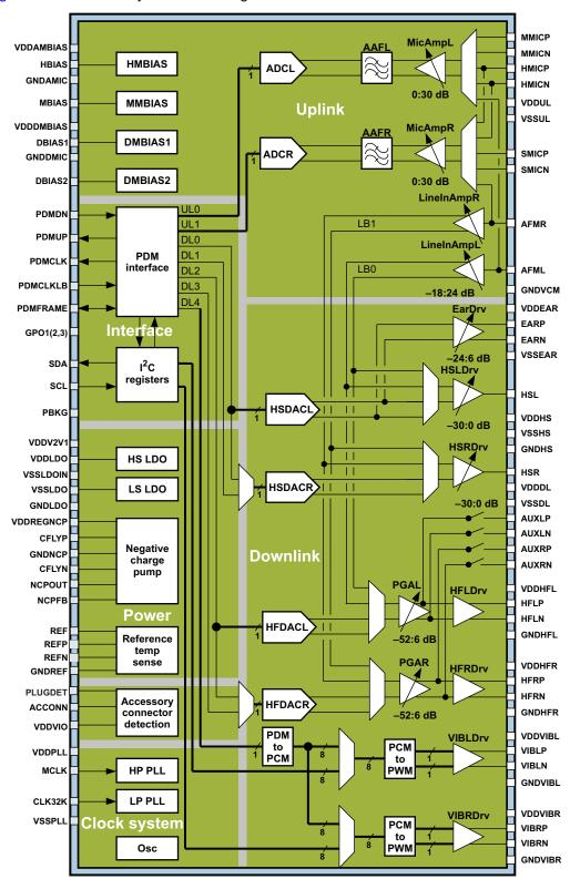
Figure 1-1. Simplified Block Diagram
