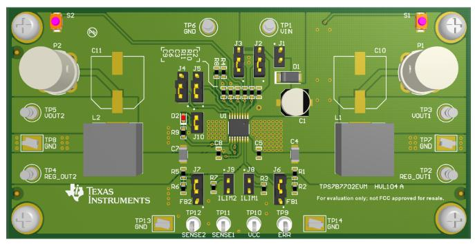
Figure 1. TPS7B7702EVM Component Placement (Assembly Top View)
