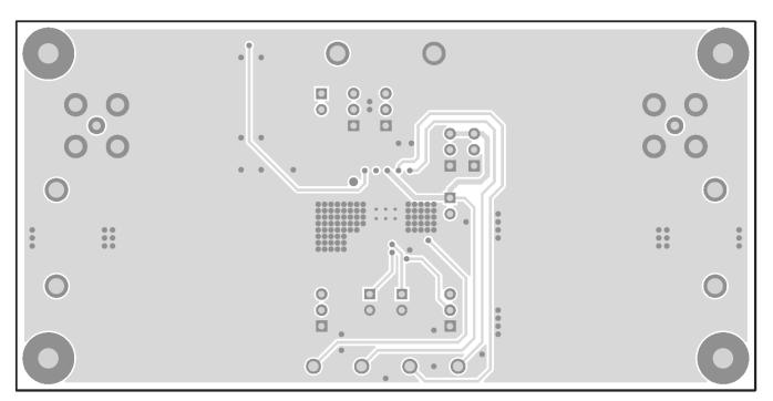
Figure 3. TPS7B7702EVM Bottom Layer Routing
