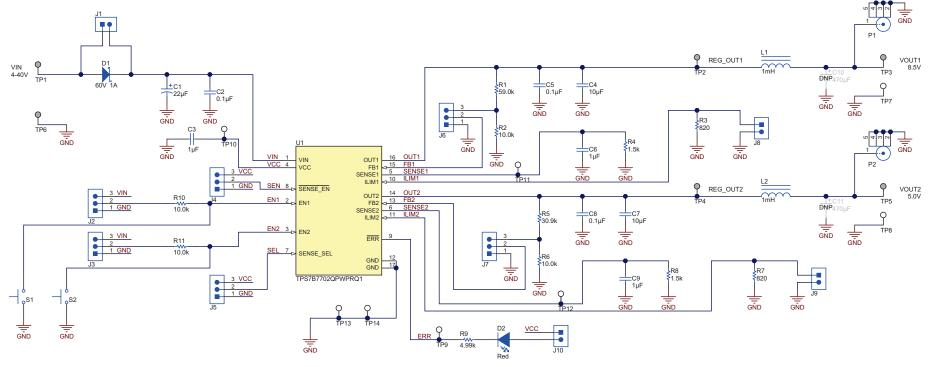
Figure 4. TPS7B7702EVM Schematic
