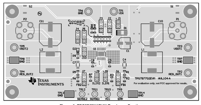
Figure 2. TPS7B7702EVM Top Layer Routing
