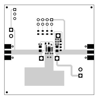
Figure 2. Top Layer Routing
