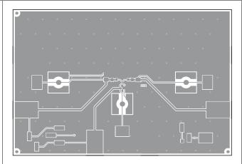
Figure 2. Top Layer Routing
