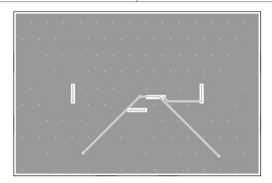
Figure 3. Bottom Layer Routing
