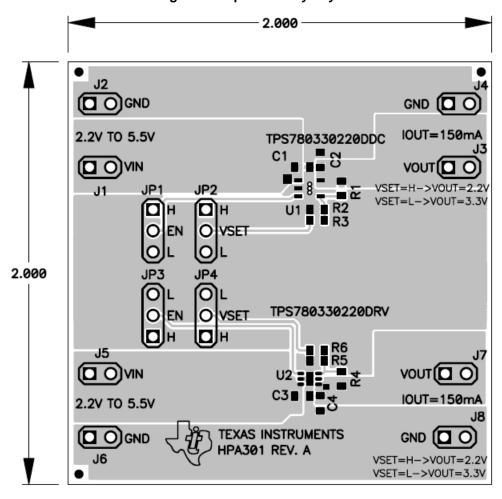
Figure 5. Top Assembly Layer
