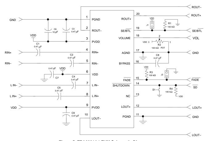
Figure 5. TPA6021A4 EVM Schematic Diagram
