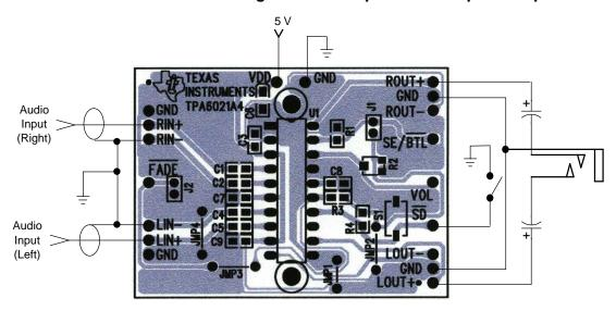
Figure 3. TPA6021A4 EVM Connected for Stereo Single-Ended Output
