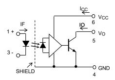
A ceramic capacitor (0.1  $\mu$ F) should be connected from pin 6 (V<sub>CC</sub>) to pin 4 (GND) to stabilize the operation of the high gain linear amplifier. Failure to provide the bypass may impair the switching property. The total lead length between capacitor and coupler should not exceed 1 cm.
