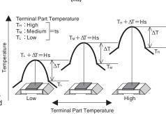
The temperature of the resistor will increase the same riangle T from the standard terminal part temperature regardlless of the ambient temperature when the same power is applied. This is because there is hardly any heat dissipation from the resistor surface to the ambient air.
