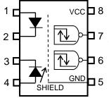
1:ANODE 1 2:CATHODE 1 3:CATHODE 2 4:ANODE 2 5:GND 6:V<sub>O</sub>2(Output2) 7:V<sub>O</sub>1(Output1) 8:V<sub>CC</sub>
