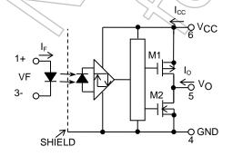
$0.1 \mu F$  bypass capacitor must be connected between pins 6 and 4
