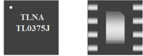
Figure 1.1 Device Image (8 Pin 2x2x0.75mm QFN Package)
