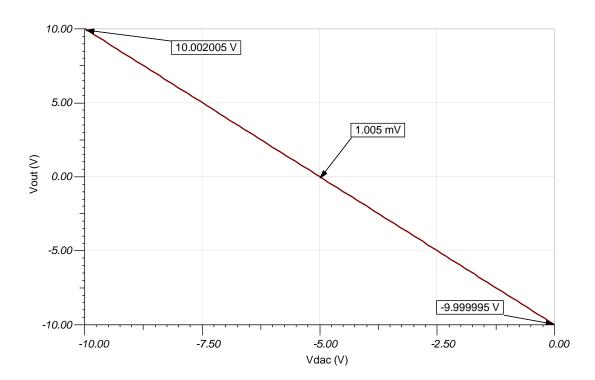
Figure 12: DAC + Transimpedance Stage, Output Transfer Function
