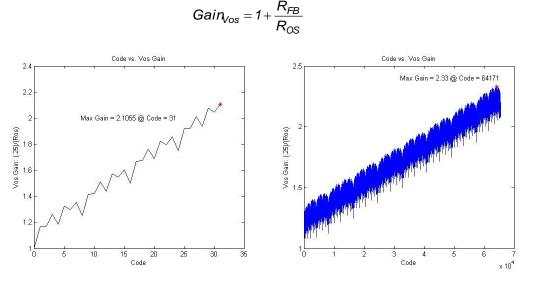
Figure 9: 5-Bit DAC, Code vs. Vos Gain
