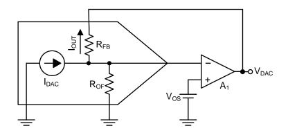
Figure 4: DAC + Transimpedance Stage Model
