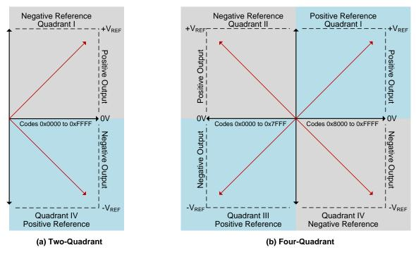
Figure 3: Two-Quadrant vs. Four-Quadrant Output
