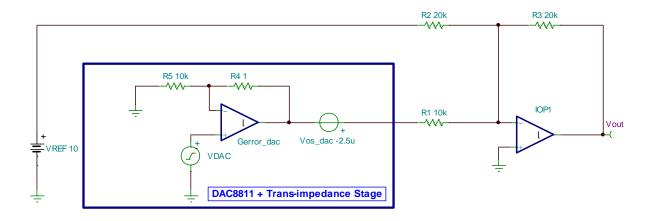
Figure 11: DAC + Transimpedance Stage Model
