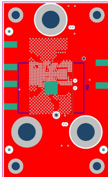
Figure 11. Bottom Components and Silk Screen Layer
