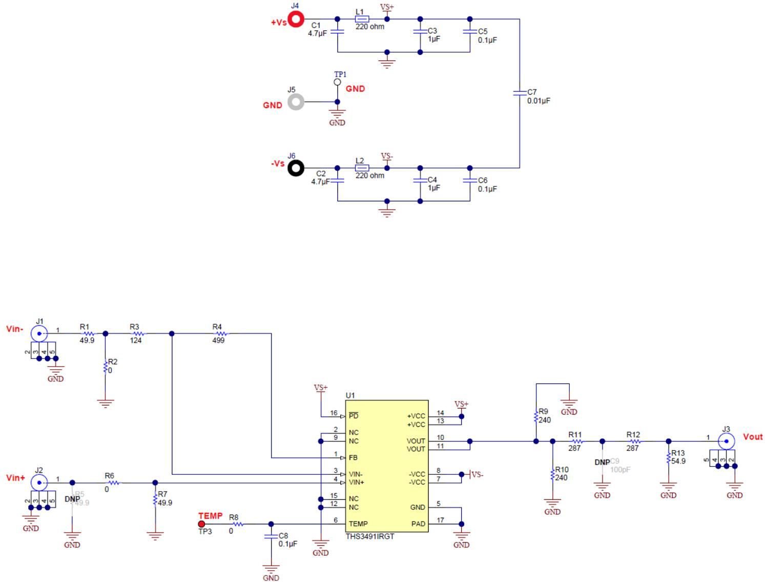
**Figure 3. Full Schematic of the THS3491RGT EVM**
