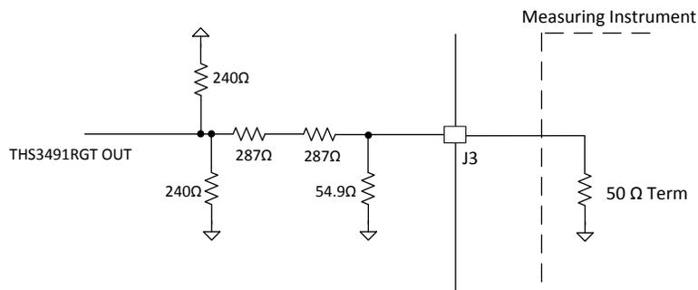
**Figure 2. Output Interface to the Measuring Instrument**
