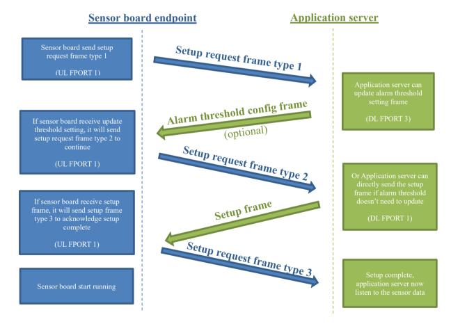
The application server can also send the update alarm threshold setting frame or the setup frame to the sensor board endpoint as a downlink message after any other uplink messages when the setting needs to be changed, and the setup process will be the same as above.
