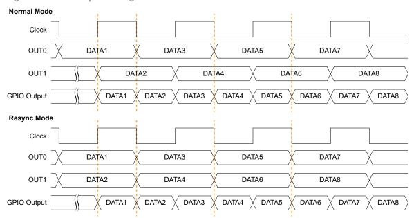
Figure 9: DDIO Output Timing Waveform
