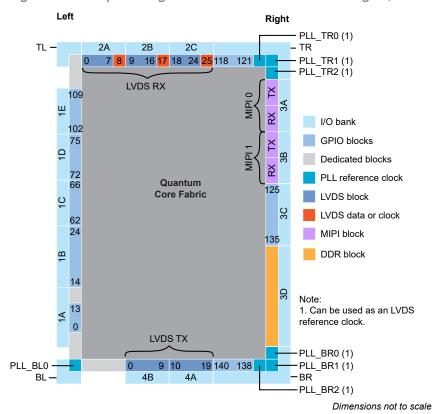
Figure 38: Floorplan Diagram for FPGAs in BGA324 Packages (with DDR and MIPI)
