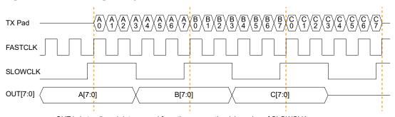
$\ensuremath{\mathsf{OUT}}$  is byte-aligned data passed from the core on the rising edge of SLOWCLK.
