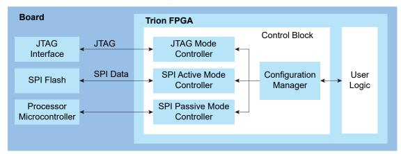
In active mode, the FPGA controls the configuration process. An oscillator circuit within the FPGA provides the configuration clock. The bitstream is typically stored in an external serial flash device, which provides the bitstream when the FPGA requests it.
