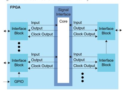
Figure 6: Interface Block and Core Connectivity
