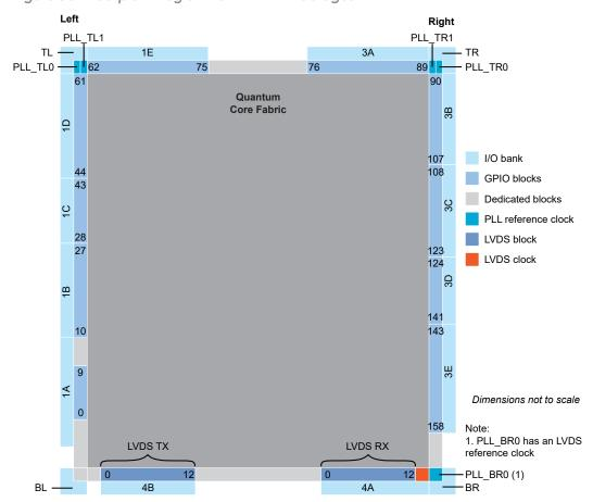
Figure 35: Floorplan Diagram for QFP144 Packages
