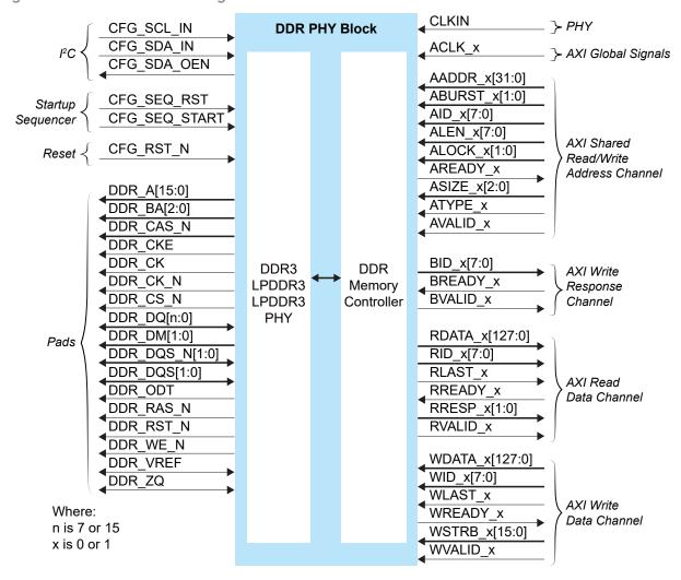
The DDR DRAM block supports an  $I^2C$  calibration bus that can read/write the DDR configuration registers. You can use this bus to fine tune the DDR PHY for high performance.
