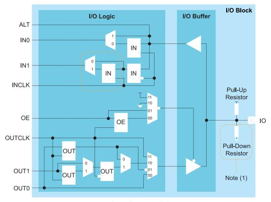
1. GPIO pins using LVDS resources do not have a pull-down resistor.
