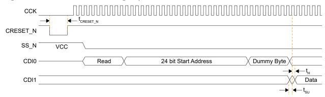
Figure 32: SPI Passive Mode (x1) Timing Sequence
