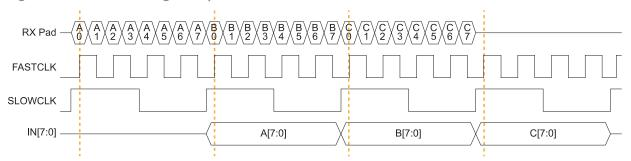
IN is byte-aligned data passed to the core on the rising edge of SLOWCLK.
