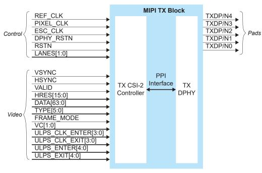
The control signals determine the clocking and how many transceiver lanes are used. All control signals are required except the two reset signals. The reset signals are optional, however, you must use both signals or neither.
