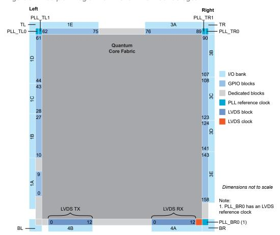
Figure 37: Floorplan Diagram for FPGAs in BGA256 Packages
