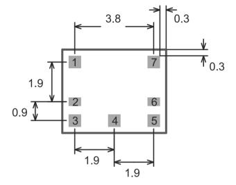
Pins 1,3,4,7 = 0.6 x 0.6 (mm) Pin 2,6 = 0.4 x 0.6 (mm)
