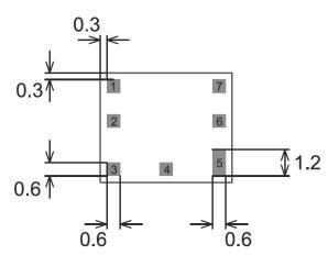
Pins 1,2,3,4,6,7 = 0.6 x 0.6 (mm) Pin 5 = 1.2 x 0.6 (mm)
