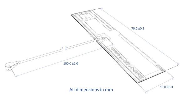
The plug connector on the antenna is an IPEX MHFI.
