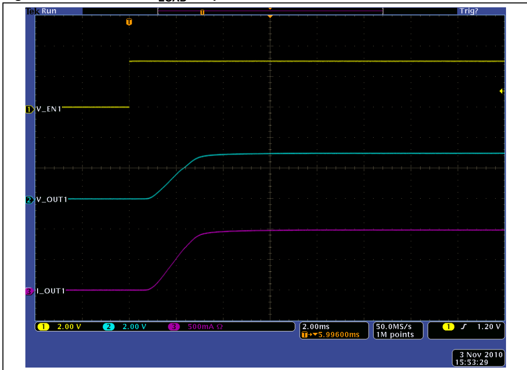
Figure 23. Turn-on for C_{LOAD} = 1\ \mu\text{F}
