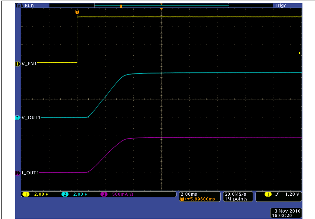
Figure 29. Turn-on for C_{LOAD} = 1 \mu F
