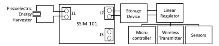
Figure 5. Example 2: Wireless sensor node with SSIM-101
