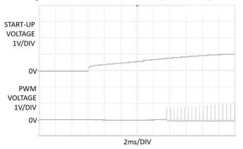
Figure 1. Start-up response of self-start controller
