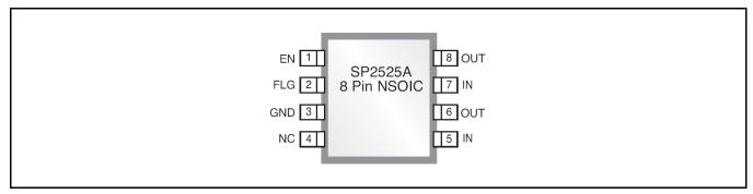
Fig. 3: SP2525A Pin Assignment
