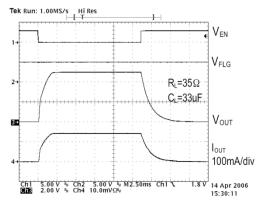
Fig. 16: Turn-On, Turn-Off Characteristics
