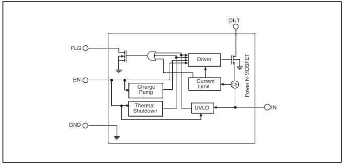
Fig. 2: SP2525A Block Diagram
