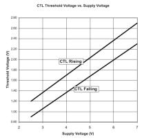
Fig. 10: CTL Threshold vs Supply Voltage
