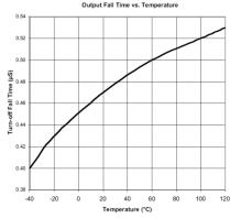
Fig. 13: Output Fall Time vs Temperature
