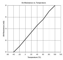
Fig. 5: Output On-Resistance vs Temperature
