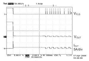
Fig. 18: Short Circuit Response (Short applied to Output)
