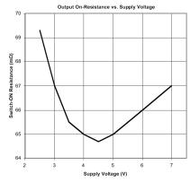
Fig. 4: Output On-Resistance vs Supply Voltage
