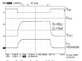
Fig. 15: Turn-On, Turn-Off Characteristics
