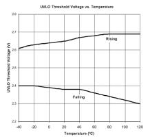
Fig. 6: UVLO Threshold vs Temperature
