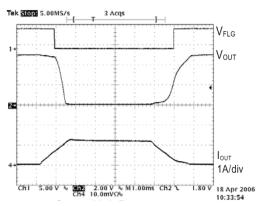
Fig. 21: Current Limit Response (Ramped Load)
