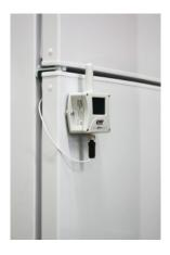
The kit includes two powerful neodymium magnets with a finish that reliably holds Datalogger including probes to magnetic metal surfaces. Connecting material included. For use with Datalogger Uxxxx.
