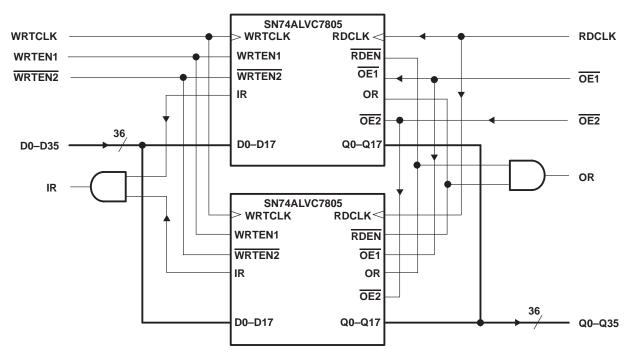
Figure 8. Word-Width Expansion:  $256 \times 36$  Bits
