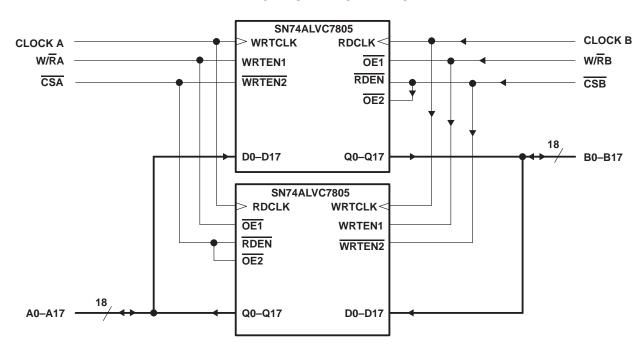
**Figure 7. Bidirectional Configuration**
