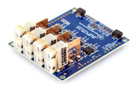
Appendix 4d: SEN-30011, Spring Clamp connector, pushbutton release, universal TC type
