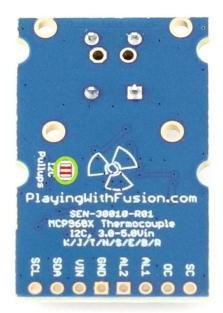
Application: one pair of pull-up resistors are required for proper I2C operation. If multiple breakouts are used together (think Qwiic daisy-chain), it is possible that an excessive amount of resistance can cause bus issues. If this is the case, resistance must be removed from one or more devices. SEN-30010 has cuttable traces on the back side of the board to make this easy.
