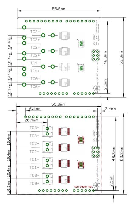
Appendix 1b: Mech Drawing, Screw Terminal (Top View)
