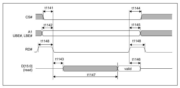
Figure 7-20: Indirect 80 Type 1 Interface Read Cycle Timing (No Wait Mode)
