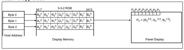
Figure 13-5: LUT Bypass for 8 Bpp mode
