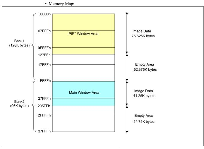
Figure 8-6: Memory Map for Main Window, PIP<sup>+</sup> Window, and Overlay Display
