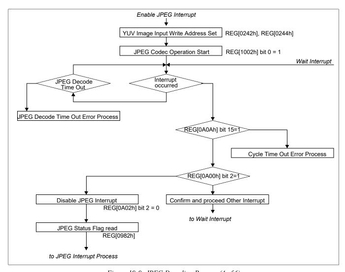
Figure 19-9: JPEG Decoding Process (4 of 6)
