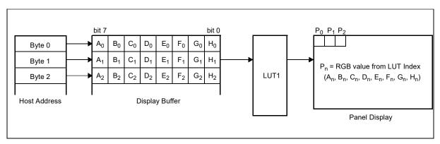
Figure 13-1: LUT1 for 8 Bpp Mode
