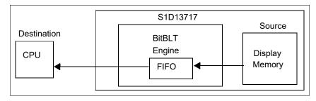
Figure 16-1: Read BitBLT Data Flow
