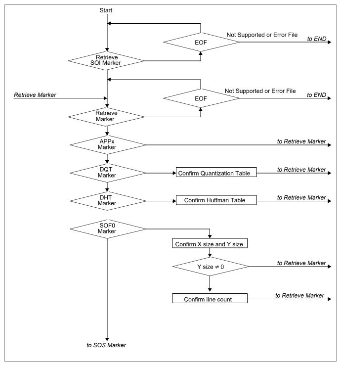
Figure 19-6: JPEG Decoding Process (1 of 6)
