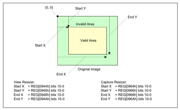
Figure 17-1: Trimming Function
