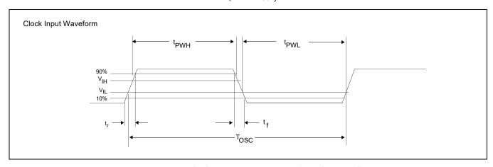
Figure 7-2: Clock Input Requirements (PLL bypassed)
