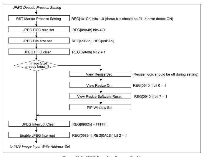
Figure 19-8: JPEG Decoding Process (3 of 6)
