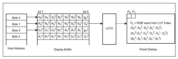
Figure 13-4: LUT2 for 16 Bpp Mode
