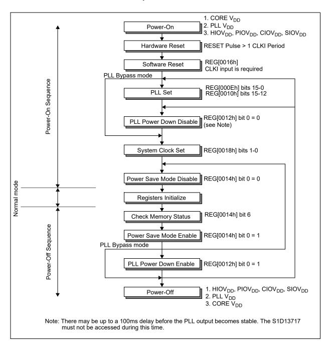
Figure 11-1: Power-On/Power-Off Sequence
