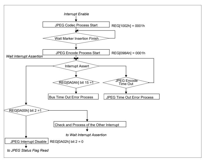
Figure 19-2: JPEG Encoding Process (1 of 4)
