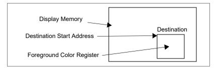
Figure 16-4: Solid Fill BitBLT Data Flow
