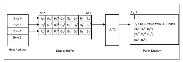
Figure 13-2: LUT2 for 8 Bpp Mode
