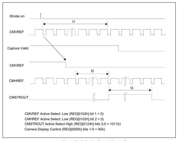
Figure 7-43: Strobe Control Output Timing
