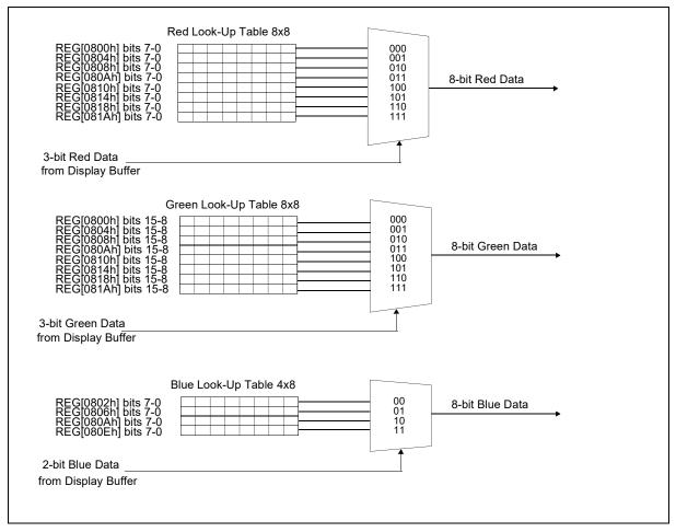
Figure 12-2: LUT2 (PIP+ Window) for 8 Bpp Architecture
