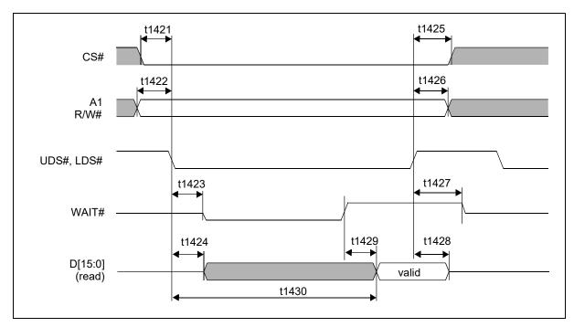
Figure 7-28: Indirect 68 Interface Read Cycle Timing (Wait Mode)
