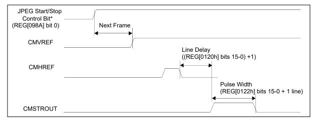
Figure 20-1: Strobe Signal Output Timing
