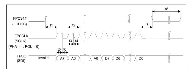
Figure 7-36: LCD1 uWIRE Serial Interface Timing
