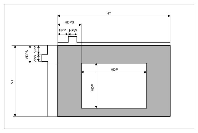
Figure 7-30: Generic TFT Panel Timing
