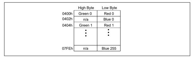
Figure 10-2: LUT1 Mapping
