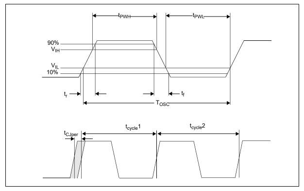
Figure 7-1: Clock Input Requirements (PLL)
