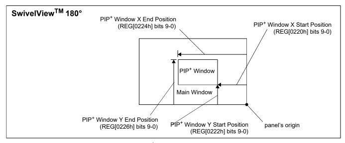
Figure 15-3: PIP<sup>+</sup> with SwivelView 180° Enabled
