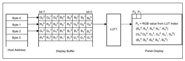
Figure 13-3: LUT1 for 16 Bpp Mode
