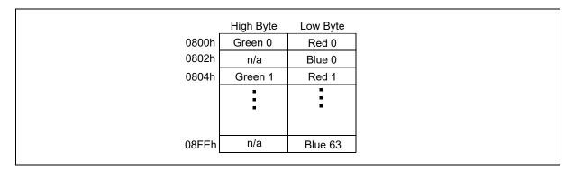
Figure 10-3: LUT2 mapping
