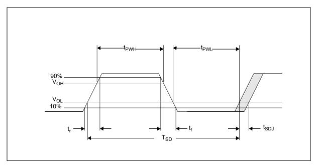
Figure 7-45: SD Memory Card Clock Output Timing
