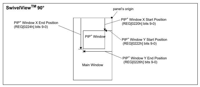
Figure 15-2: PIP<sup>+</sup> with SwivelView 90° Enabled
