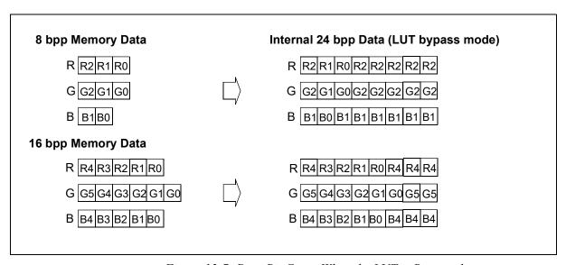
Figure 13-7: Data Bit Cover When the LUT is Bypassed
