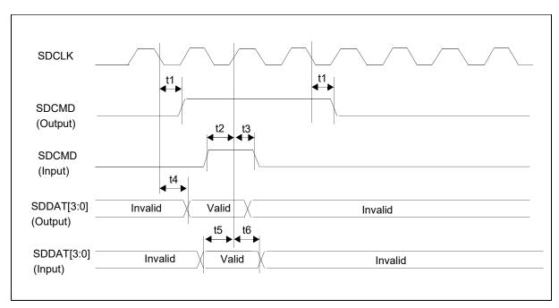
Figure 7-44: SD Memory Card Access Timing
