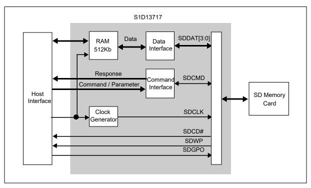
Figure 21-1: SD Memory Card Interface Block Diagram
