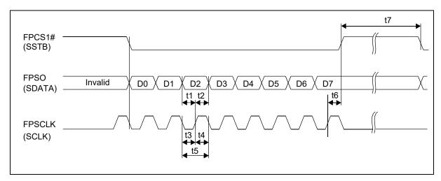
Figure 7-35: LCD1 a-Si TFT Serial Interface Timing
