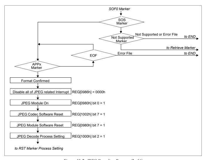
Figure 19-7: JPEG Decoding Process (2 of 6)
