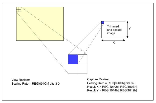
Figure 17-2: Scaling Example (1/2 Scaling)
