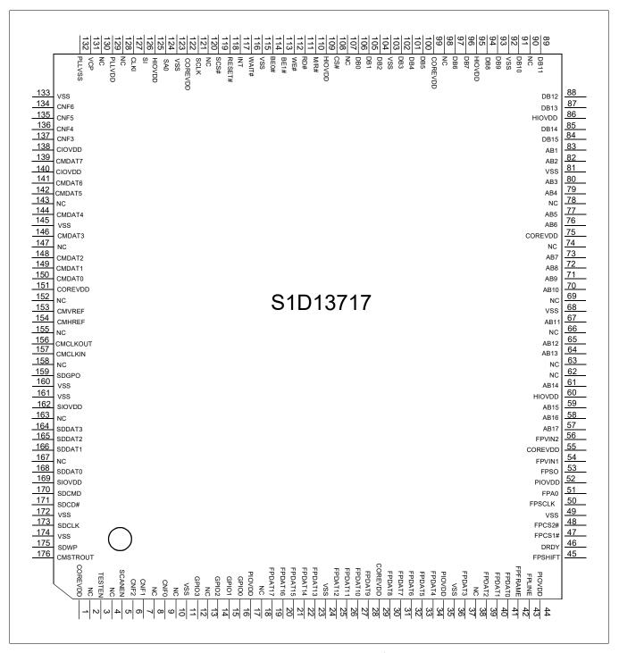
Figure 5-1: S1D13717 QFP21 176-Pin Package - Top View
