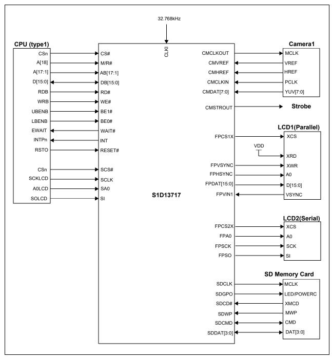
Figure 3-3: S1D13717 System Diagram 3
