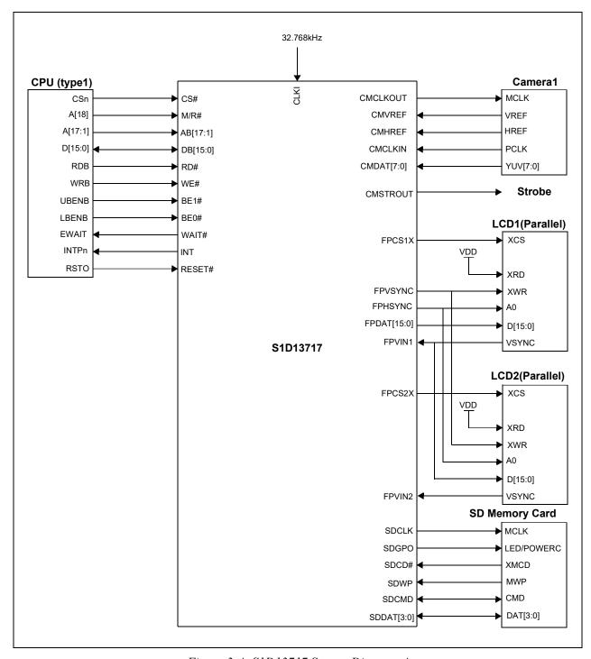
Figure 3-4: S1D13717 System Diagram 4
