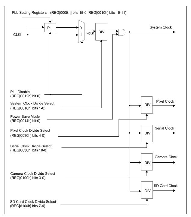
Figure 9-1: Clock Diagram
