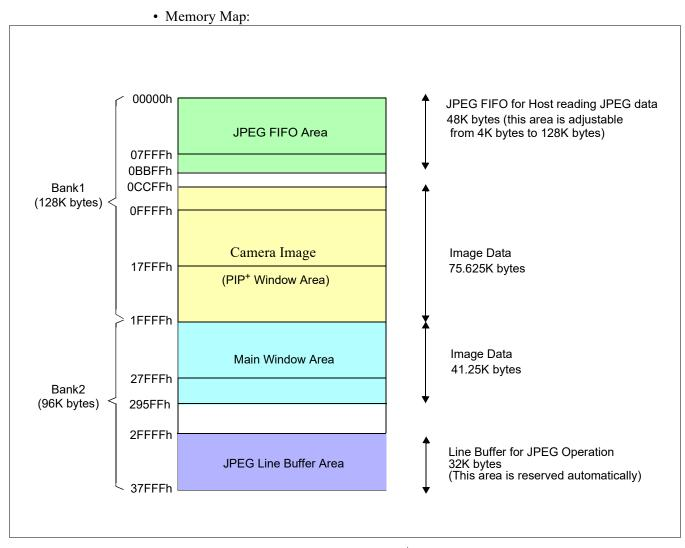
Figure 8-10: Memory Map for Main Window, PIP+ Window, Overlay and JPEG
