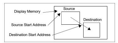
Figure 16-2: Move BitBLT data flow
