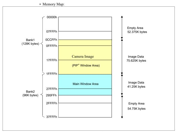
Figure 8-8: Memory Map for Main Window, PIP<sup>+</sup> Window, Overlay, and YUV
