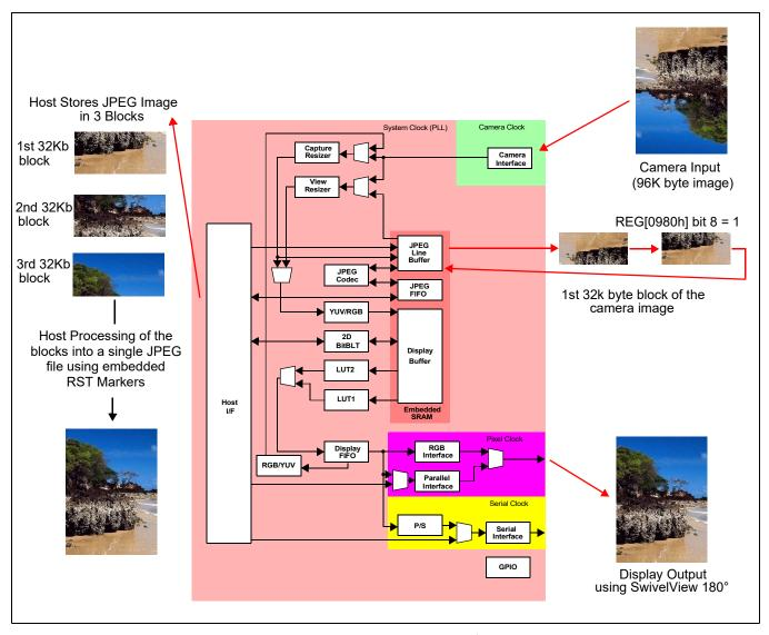
Figure 18-5: JPEG 180° Rotate Encode Diagram
