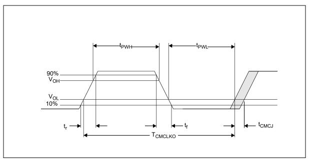
Figure 7-42: Camera Clock Output Timing
