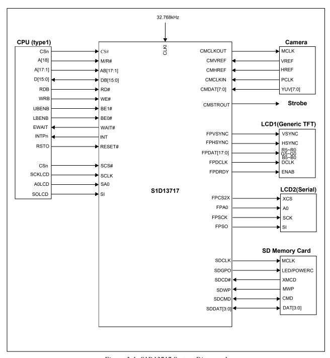
Figure 3-1: S1D13717 System Diagram 1
