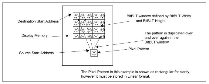
Figure 16-3: Pattern Fill Drawing
