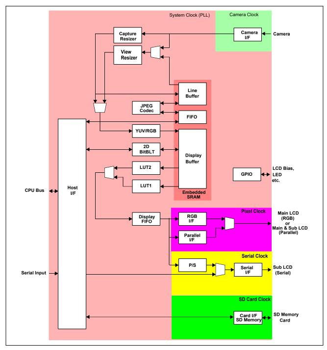
Figure 4-1: S1D13717 Block Diagram
