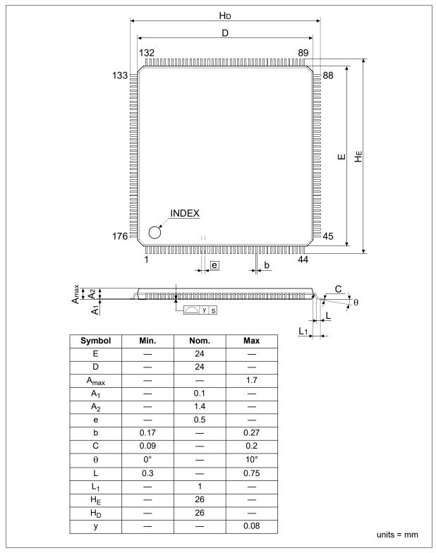
Figure 23-1: S1D13717 QFP21-176 Pin Package
