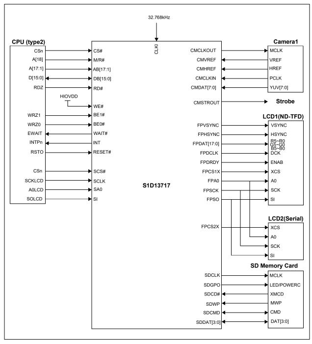
Figure 3-2: S1D13717 System Diagram 2
