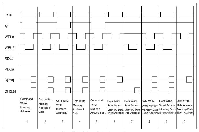
Figure 22-2: Memory Write Example Sequence
