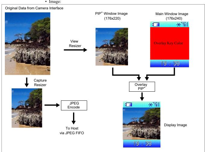
Figure 8-9: Main Window, PIP+ Window, Overlay, and JPEG
