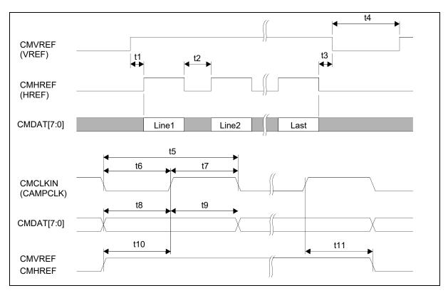
Figure 7-41: Camera Interface Timing
