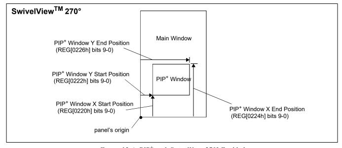
Figure 15-4: PIP<sup>+</sup> with SwivelView 270° Enabled
