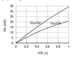
Vol vs. Iol (INTR pin) (VIN=VDD, Topt=25°C)
