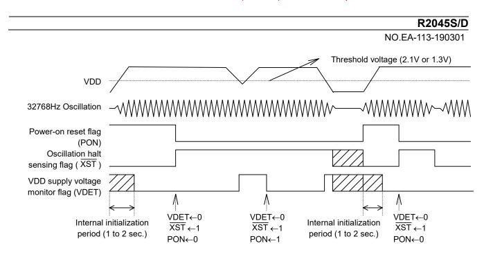
When the PON bit is set to 1 in the control register 2, the DEV, F6 to F0, WALE, DALE,  $\overline{12}$  /24,  $\overline{\text{CLEN2}}$ , TEST, CT2, CT1, CT0, VDSL, VDET,  $\overline{\text{CLEN1}}$ , CTFG, WAFG, and DAFG bits are reset to 0 in the oscillation adjustment register, the control register 1, and the control register 2. The PON bit is also set to 1 at power-on from 0 volts.
