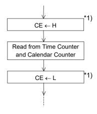
\*1) When reading clock and calendar counters, do not drive CE to L until all times from second to year have been written to prevent error in writing time. For more detailed in "Considerations in Reading and Writing Time Data under special condition".
