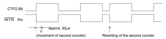
In the pulse mode, the increment of the second counter is delayed by approximately 92  $\mu$ s from the falling edge of clock pulses. Consequently, time readings immediately after the falling edge of clock pulses may appear to lag behind the time counts of the real-time clocks by approximately 1 second. Rewriting the second counter will reset the other time counters of less than 1 second, driving the  $\overline{\text{INTR}}$  pin low.
