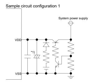
\*1) Install bypass capacitors for high frequency and low frequency applications in parallel in close vicinity to the R2045S/D.
