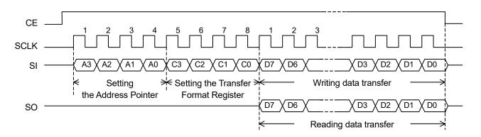
Two types of data transfer formats are available for reading data transfer and writing data transfer each.
