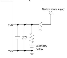
\*1) When using an OR diode as a power supply for the R2045S/D ensure that voltage exceeding the absolute maximum rating of VDD+0.3v is not applied the SO pin.
