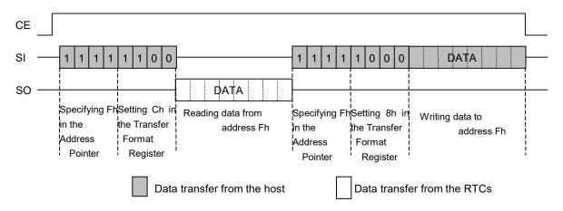
The reading and writing data transfer formats correspond to the settings in the transfer format register as shown in the table below.
