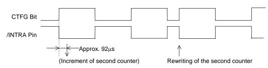
In the pulse mode, the increment of the second counter is delayed by approximately 92  $\mu$ s from the falling edge of clock pulses. Consequently, time readings immediately after the falling edge of clock pulses may appear to lag behind the time counts of the real-time clocks by approximately 1 second. Rewriting the second counter will reset the other time counters of less than 1 second, driving the /INTRA pin low.
