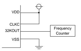
\* 1) When power-on, the R2025S/D is configured to generate 32.768-kHz clock pulses for output from the 32KOUT pin.
