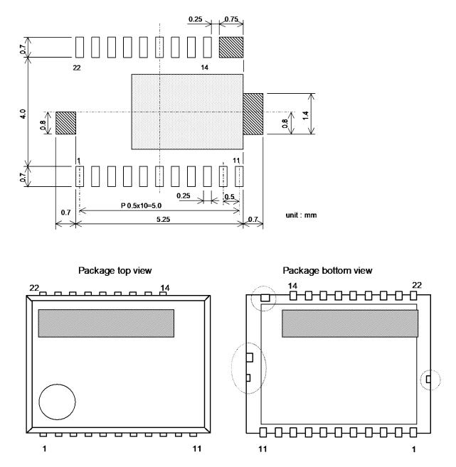
1. Pad layout and size can modify by customers material, equipment, and method. Please adjust pad layout according to your conditions.
