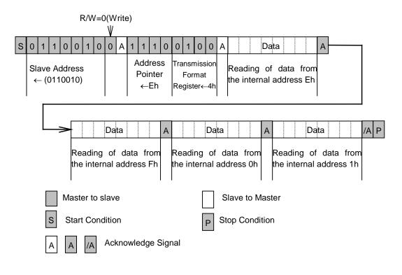
The third method to reading data from the internal register is to start reading immediately after writing to the Slave Address and R/W bit. Since the Internal Address Pointer is set to Fh by default as described in the first method, this method is only effective when reading is started from the Internal Address Fh.
