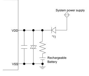
\*1) Install bypass capacitors for high-frequency and low-frequency applications in parallel in close vicinity to the R2025S/D.
