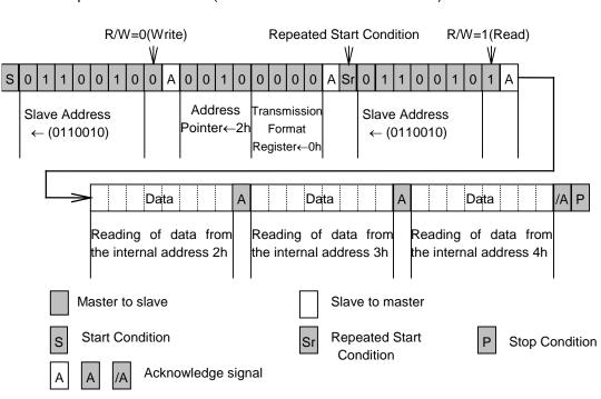
The second method to reading data from the internal register is to start reading immediately after writing to the Internal Address Pointer and the Transmission Format Register. Although this method is not based on I<sup>2</sup>C-Bus standard in a strict sense it still effective to shorten read time to ease load to the master. Set 4h to the transmission format register when this method used.
