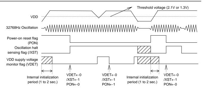
When the PON bit is set to 1 in the control register 2, the DEV, F6 to F0, WALE, DALE, /12·24, /CLEN2, TEST, CT2, CT1, CT0, VDSL, VDET, /CLEN1, CTFG, WAFG, and DAFG bits are reset to 0 in the oscillation adjustment register, the control register 1, and the control register 2. The PON bit is also set to 1 at power-on from 0 volts.
