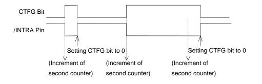
\*1), \*2) When the oscillation adjustment circuit is used, the interrupt cycle will fluctuate once per 20sec. or 60sec. as follows:
