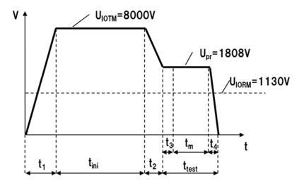
$t_1$ ,  $t_2$  = 1 to 10 sec  $t_3$ ,  $t_4$  = 1 sec  $t_m$  (PARTIAL DISCHARGE) = 10 sec  $t_{test}$  = 12 sec  $t_{ini}$  = 60 sec
