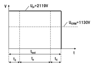
$t_3$ , $t_4$ =0.1 sec  $t_p$  (PARTIAL DISCHARGE) = 1.0 sec  $t_{test}$ =1.2 sec
