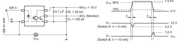
C∟ includes probe and stray wiring capacitance.
