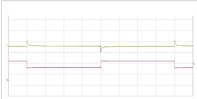
Output voltage response to load current step- change (1.66-2.49-1.66 A) at: T_{P1} = +25^{\circ}\text{C} , V_i = 48\text{ V} . Top trace: output voltage (500 mV/div.). Bottom trace: load current (1 A/div.). Time scale: (2 ms/div.).
