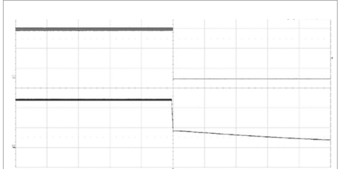
Shut-down enabled by disconnecting V_I at: T_{P1} = +25^\circ\text{C} , V_I = 48\text{ V} , I_O = 6\text{ A} resistive load. Top trace: output voltage (2 V/div.). Bottom trace: input voltage (20 V/div.). Time scale: (200 ms/div.).
