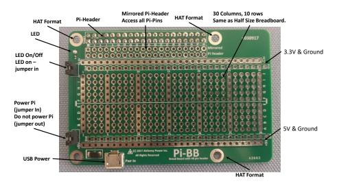
Pi-BB is a powered breadboard designed for the Raspberry Pi. Pi-BB offers the following features:
