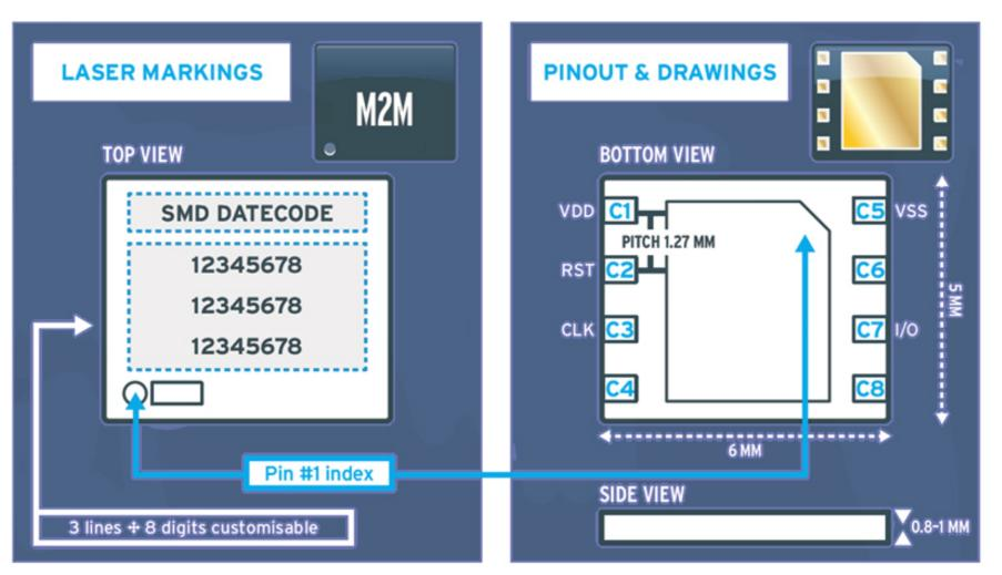
The SMD can be laser marked with up to 10 characters x 3 lines. For eye readability we recommend not exceeding 8
